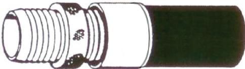
**Important:** Please note the mender threads are different on each end. One is left hand and one is right hand. Screw the mender about 2/3rds into the end of the tube using a wrench on the center knurled shoulder. Then unscrew it. Repeat the procedure for the other end. Watch for the left hand thread.
